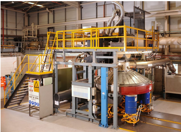
Fig. 12 The semi-industrial scale (3 m in diameter) integrated heat recovery and dry granulation pilot plant at CSIRO [40] (color figure online)
