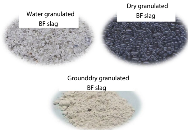
Fig. 14 Samples of wet and dry granulated iron blast furnace slag [39] (color figure online)
