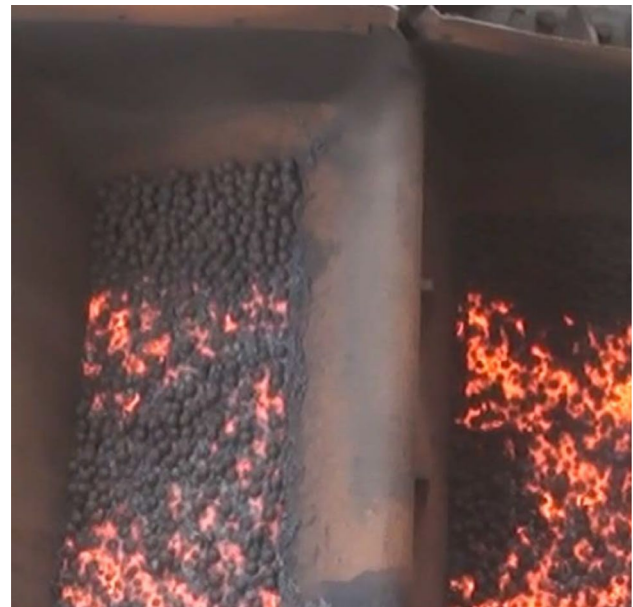
Fig. 15 Paul Wurth's dry granulation pilot plant—cooling of slag with steel spheres in the mould [48] (color figure online)
