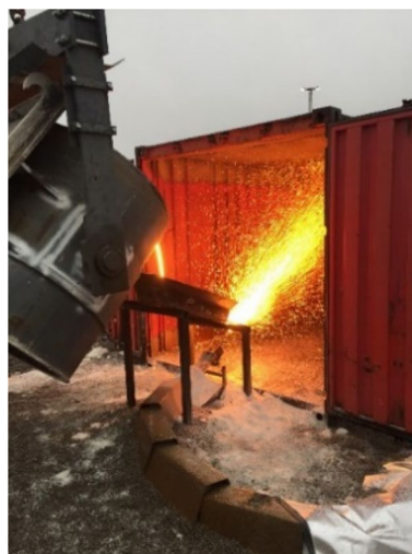
Fig. 4 Photograph of onsite pilot-scale air granulation testing at SMT (Color figure online)
