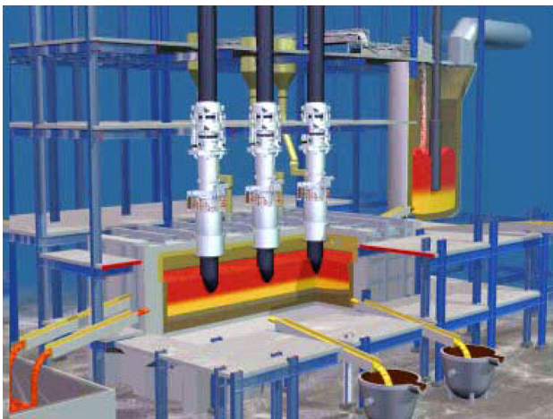
Fig. 4 3D illustration of a rectangular slag-cleaning furnace [19] (Color figure online)
