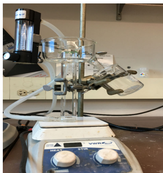
Fig. 3 The Partridge-Smith cell set-up
