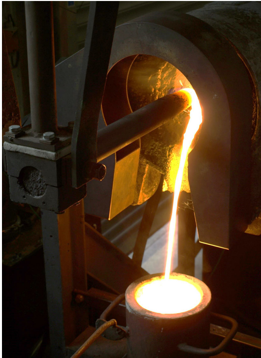
Fig. 8 Tapping of the slag from the small scale EAF
