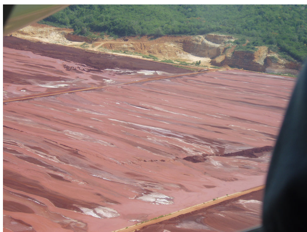
Fig. 5 Mud dewatering and compaction, Ewarton, Jamaica
