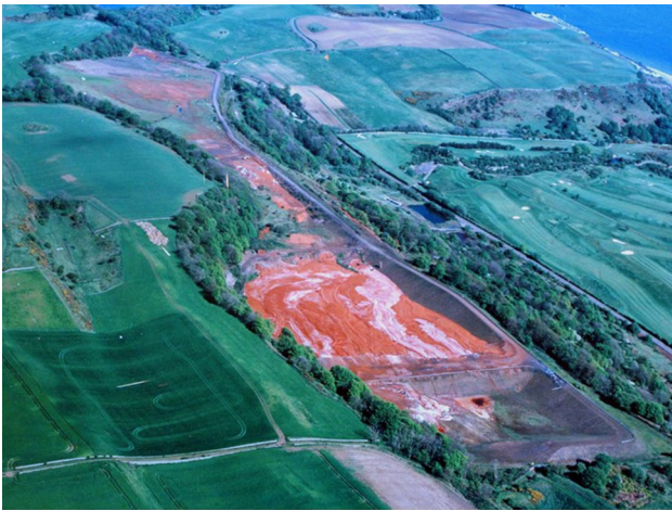
Fig. 2 Bauxite residue disposal into a former oil shale mine, Whinnyhall, Scotland
