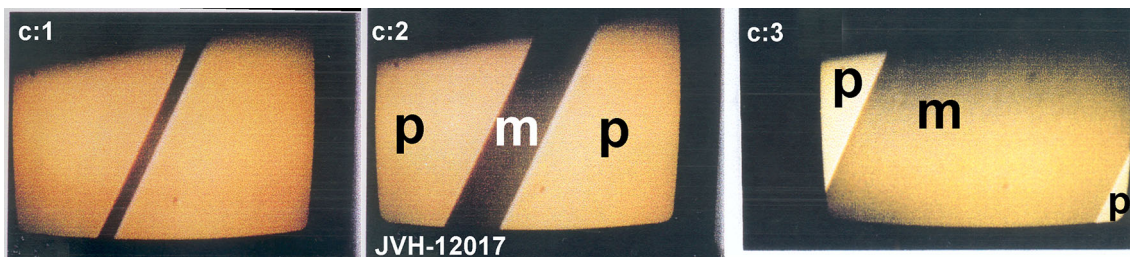
Fig. 3 Thermoelasticity in Cu–Zn–Al, single crystal: interface displacements on cooling (c), respectively (c:1, c:2 and c:3, at 287.15, 285.29 and 285.15 K). In the screen, the sample length was near 1 \text{ mm}
