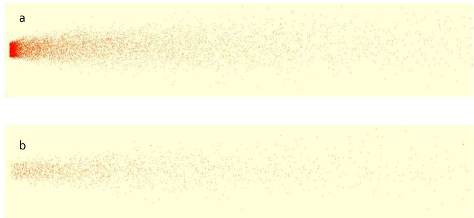
Fig. 32 Simulation of the impact of degradation upon a contaminant plume. The conditions for the simulations in the upper ( a ) and lower ( b ) diagrams are the same as those in Fig. 31 with the exception that assumed degradation rate constant is set equal to 0.01 \text{ t}^{-1} where t is the simulation time unit
