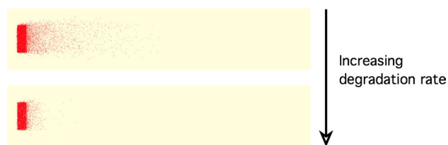
Fig. 22 Impact of degradation upon the size of the contaminant plume
