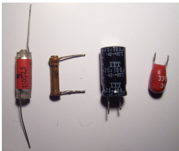
Fig. 5 Examples of dielectric capacitors with plastic foil dielectric, oxide insulator, electrolytic capacitor with aluminum and tantalum electrodes (left to right)
