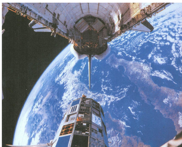
Fig. 6 Recovery of the LDEF experiment from LEO. The open space shuttle is ready to receive the LDEF cylinder
