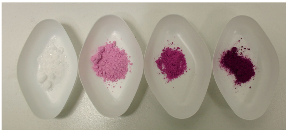
Fig. 3 Mixed crystals of K(\text{ClO}_4)_{1-x}(\text{MnO}_4)_x . From left to right: x = 0.0000 , 0.0004 , 0.0030 , and 0.0100
