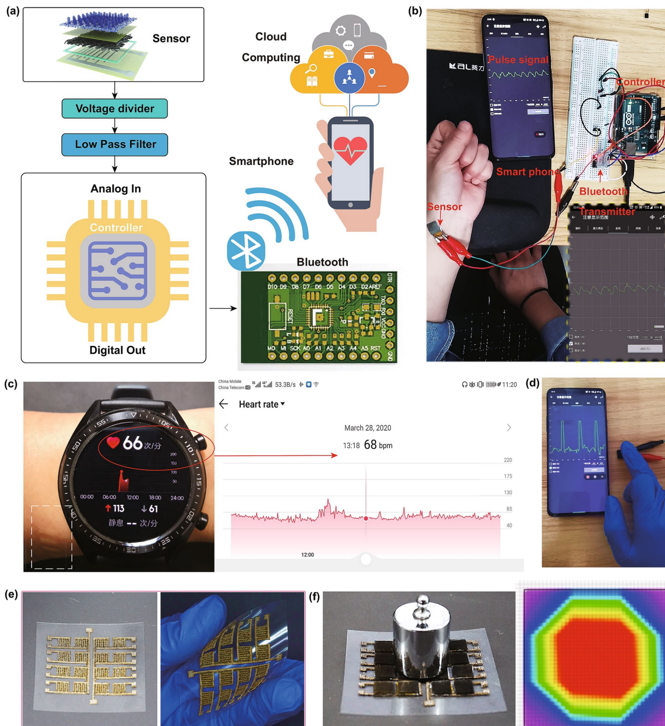
Fig. 6 Wireless real-time pulse monitoring of the sensor for healthcare. a Device configuration of the wearable sensor system. b Practical application of detecting the pulse wave and successfully send the signal to the smartphone. c Commercial sports watch showed a similar date value collected by our wearable sensor. d Practical application of gentle touching. e 4 \times 4 sensor array and its corresponding highly flexible circuit diagram. f Pressing geometrical area of the weight measured by the sensor array
