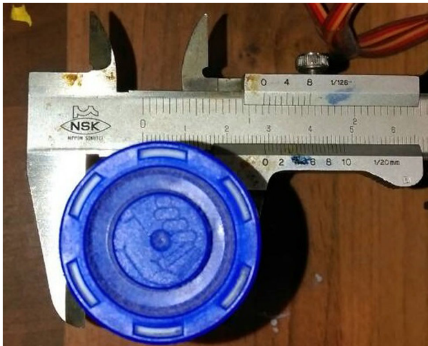
Fig. 20 Real width of the grasped object (Case 3)
