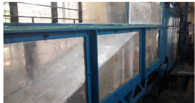
Fig. 2 Experimental flume setup for \theta = 17.6^\circ
