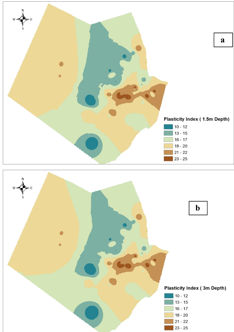
Fig. 4 Spatial variation of plasticity index with depth: a 1.5 m, b 3 m, c 4.5 m, d 6 m
