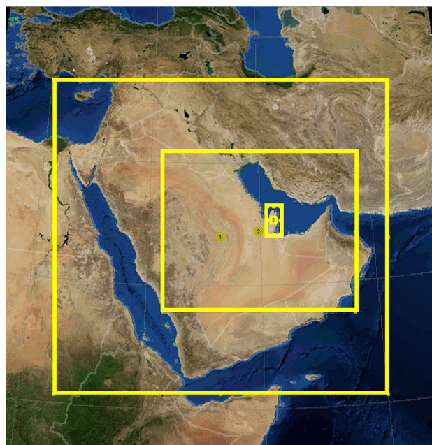
Fig. 1 Modeling domain of WRF-Chem for the Middle East in a triple nested configuration
