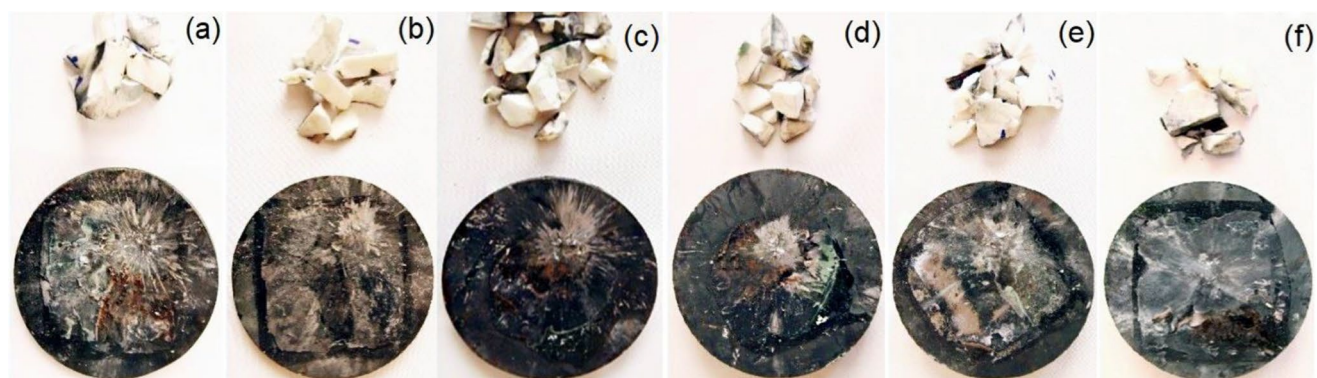
Fig. 11 The particles of broken alumina ceramic tile and successful bainitic steel layer of alumina/BS samples after the ballistic test (a) A1, (b) A2, (c) A3, (d) A4, (e) A5, (f) A6
