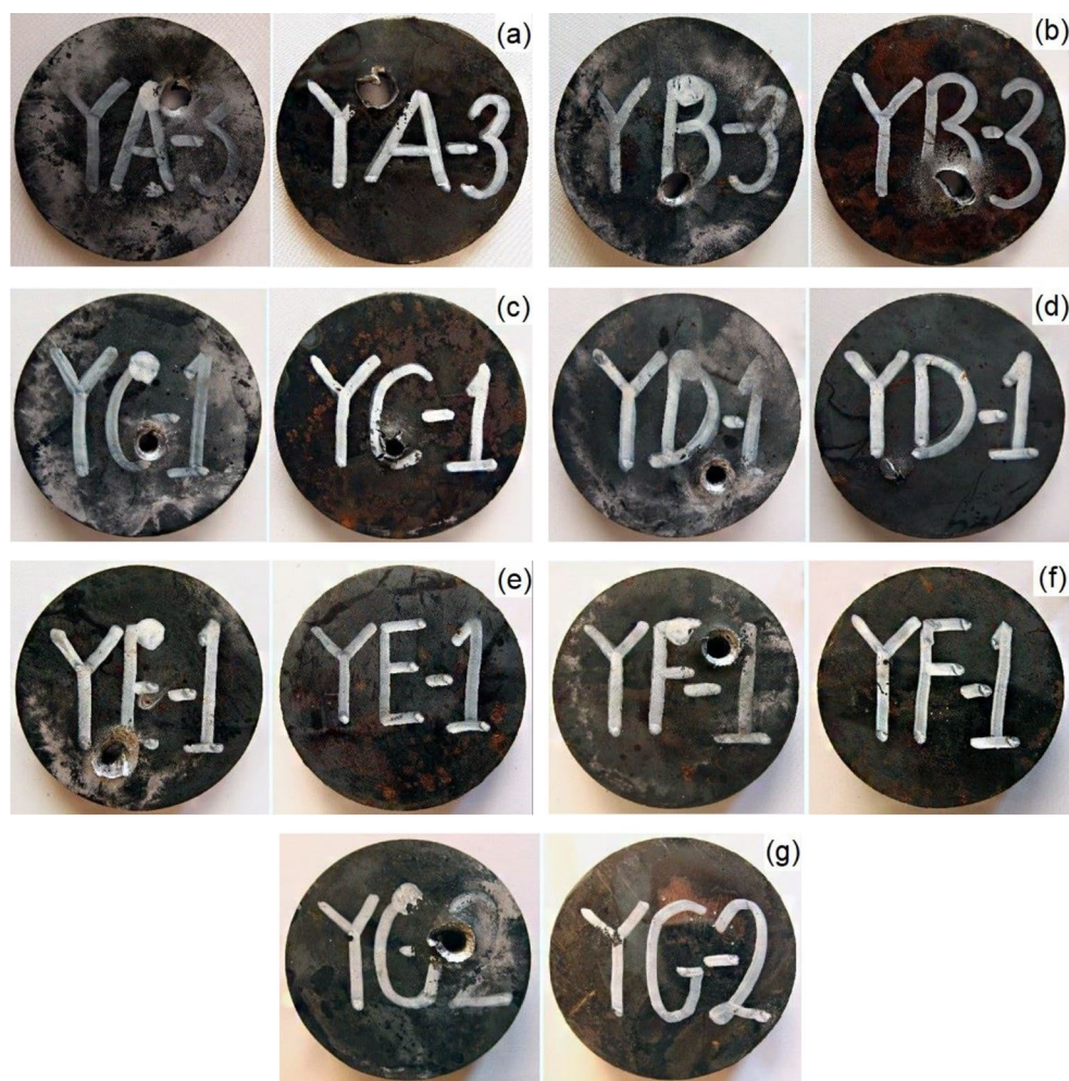
Fig. 7 The front and back views of BS samples after the ballistic shot (a) B0, (b) B1, (c) B2, (d) B3, (e) B4, (f) B5, (g) B6
