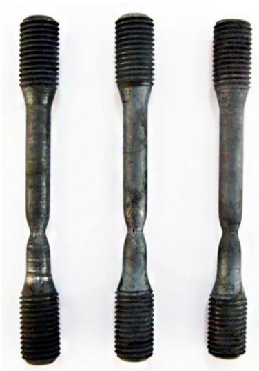
Fig. 4 Tensile specimens of bainitic steel after the tensile testing
