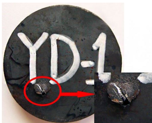
Fig. 8 Radial crack formation at the rear side of B3
