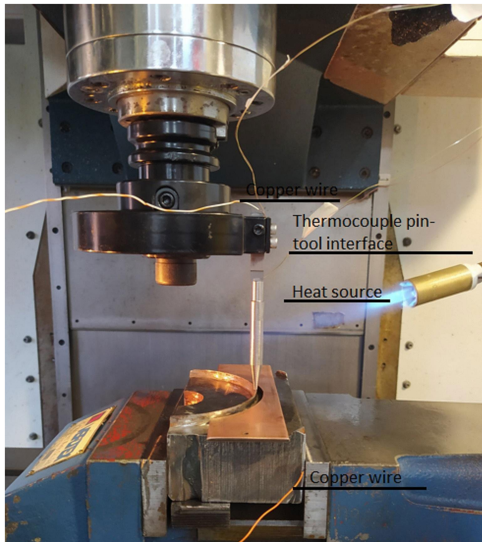
Fig. 2 Calibration setup for the tool-workpiece thermocouple
