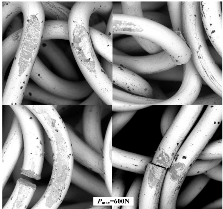
Fig. 16 SEM observed result of metal wire component with P_{\max} fixing at 600 N and N at 10 million
