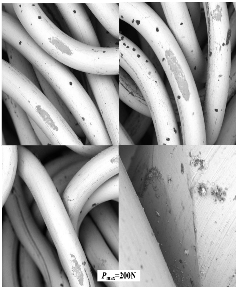
Fig. 14 SEM observed result of metal wire component with P_{\max} fixing at 200 N and N at 10 million
