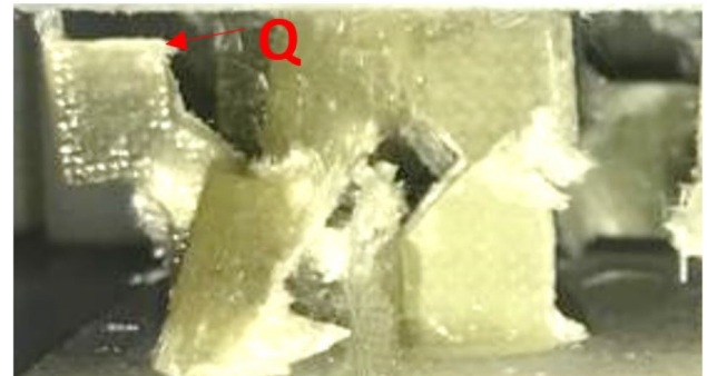
Fig. 12 Compression test of Fiber glass sandwich panel and the structure collapses from point Q region
