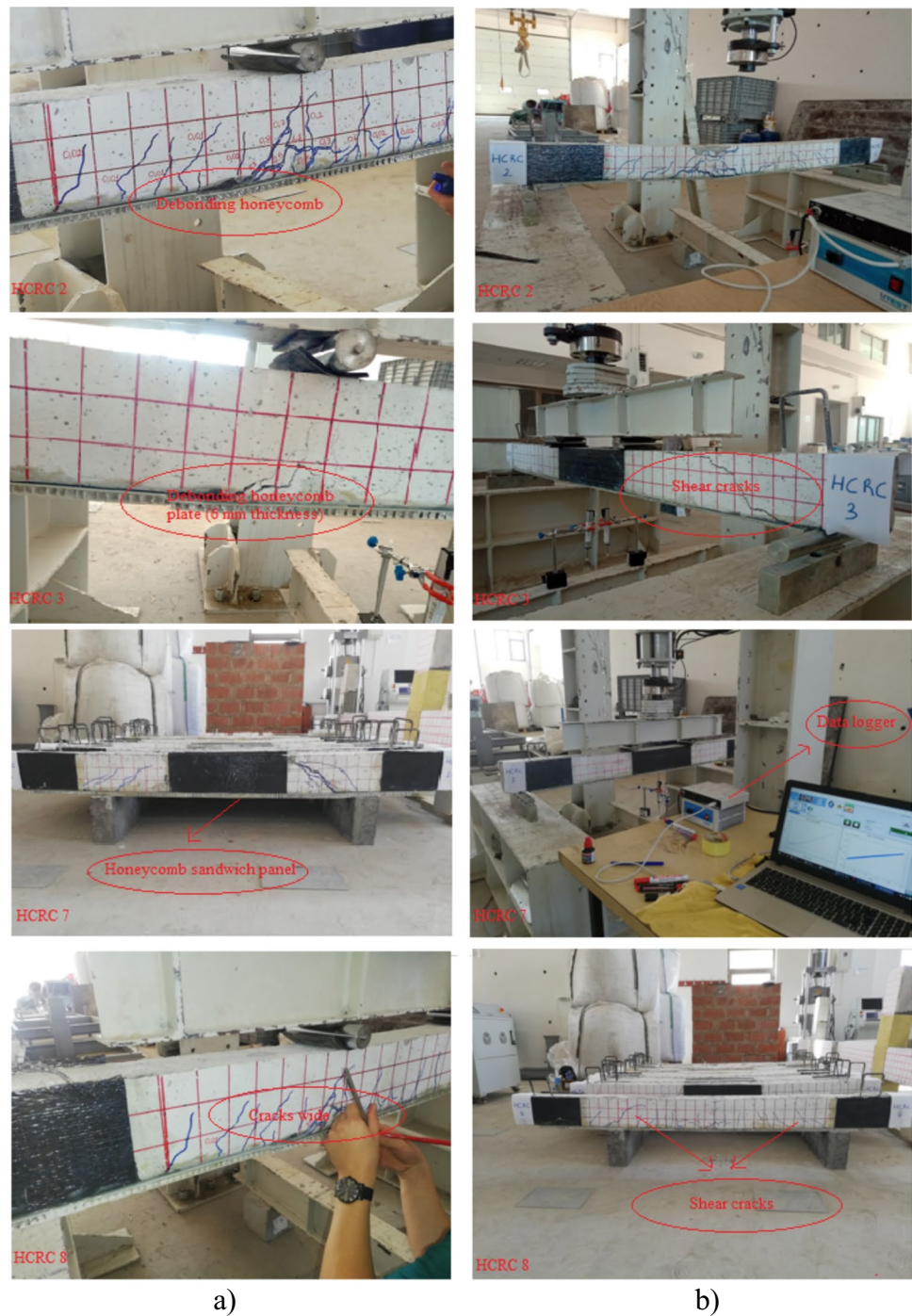
Fig. 12 The crack pattern for RC beam specimens: (a) Close up of RC beams; (b) Complete look of RC beams
