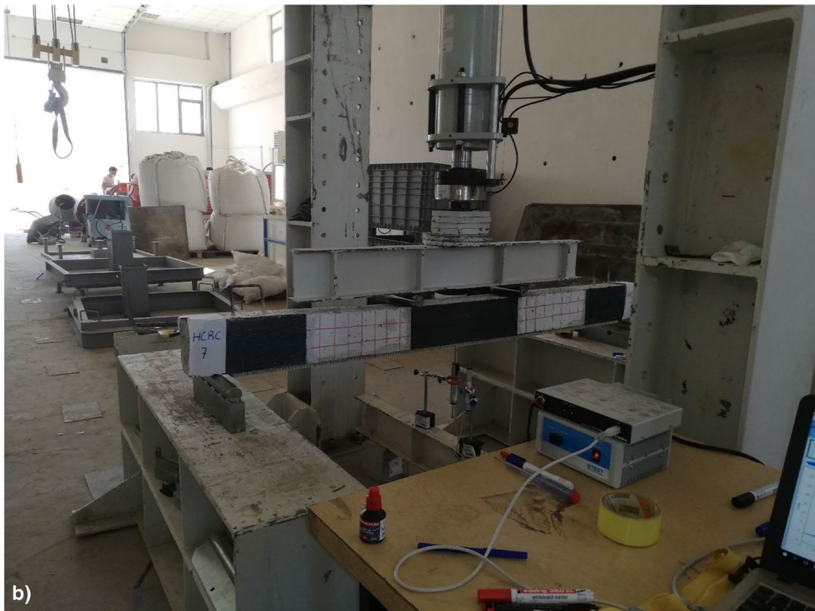
Fig. 8 (a) Front view (frame system), (b) Testing procedures (four-point bending)
