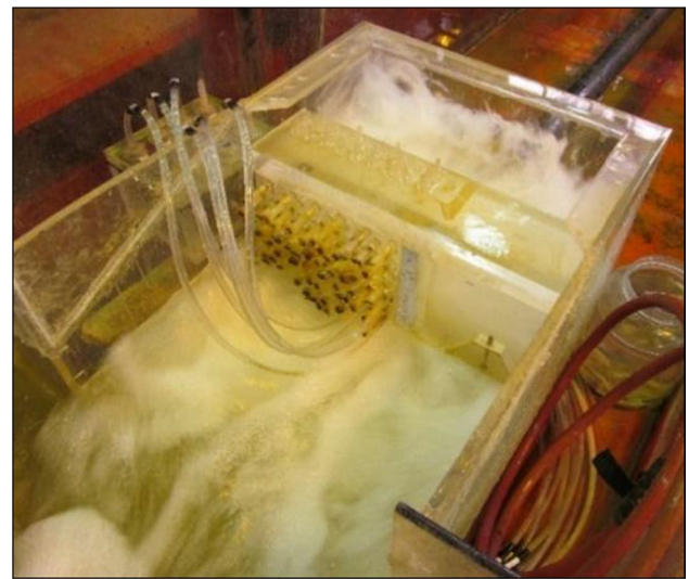
Fig. 5 Physical model of USBR VI stilling basin [47]
