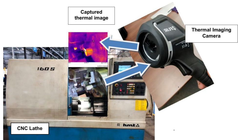
Fig. 3 Experimental setup and thermal image capturing
