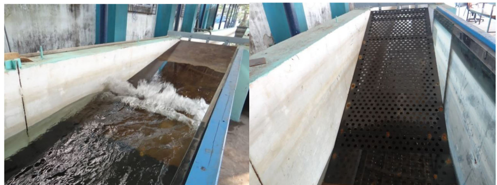
Fig. 2 View of single inclined plate model arranged inside the wave flume
