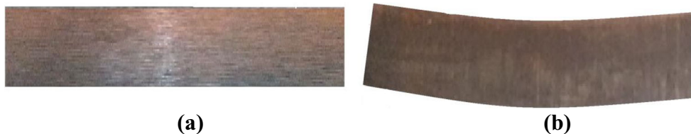
Fig. 3 Effects of heat treatment on dimensional quality of samples (a) Well dimensional sample (b) Failed sample
