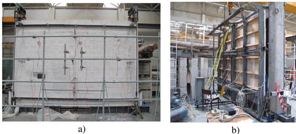
Fig. 3 – General view of the OOP experimental test set-up: (a) front view, (b) near view
