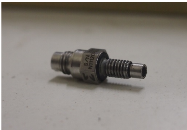
Fig. 2 A sample of the piezoresistive transducer used in the experiments
