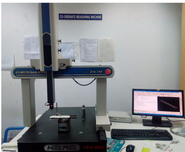
Fig. 3 Measurement of test specimen dimensions using co-ordinate measuring machine with Geomet software
