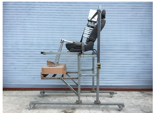
Fig. 6 Sled with the testing ATD
