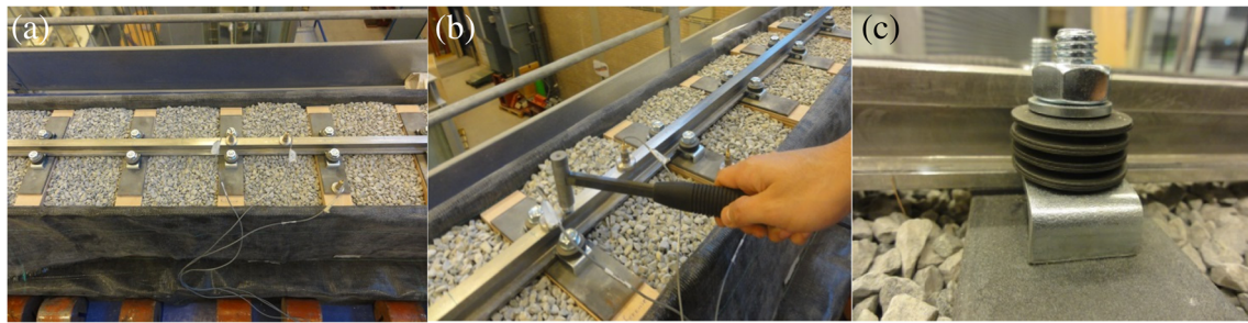
Fig. 13 a A 1:5 downscale ballasted railways track; b hitting the rail surface using an instrumented impact hammer; c magnified view of the designed fastening system for fixing the rail on sleepers
