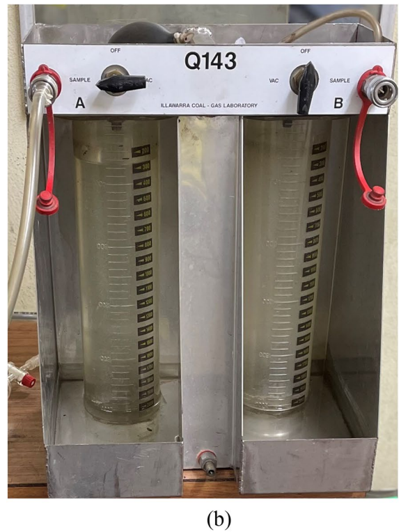
Fig. 1 Lost gas content ( Q_1 ) calculation illustration a and its measuring apparatus b (Australia 2016)
