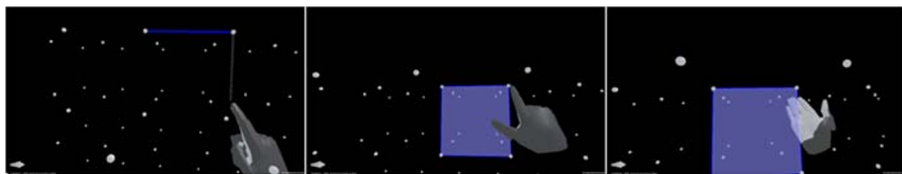
Fig. 17 Gesture-based operators in LatticeLand: a how to point to inscribe segments; b how to use a backwards “L” gesture to inscribe polygonal faces; c how to use a hand swipe to erase
