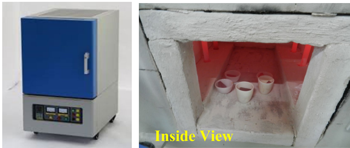
Fig. 2 Test setup-oxidation and corrosion test (IFC make)
