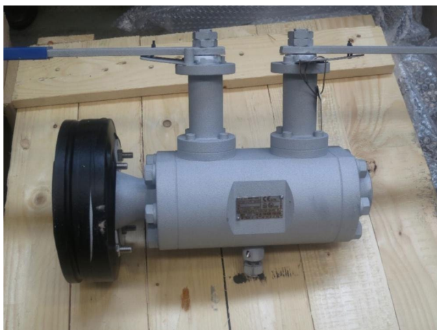
Fig. 4 A modular valve coated with TSA for offshore use (photograph by author)
