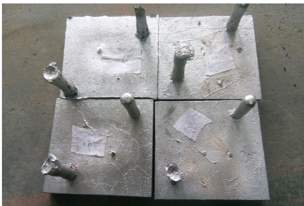
Fig. 3 Prepared Al-A356—hematite composite with Copper chills
