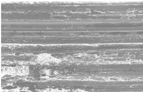
Fig. 3 SEM micrograph of hypereutectoid steel, Speed-7 m/s, Normal Pr. 0.8749 MPa
