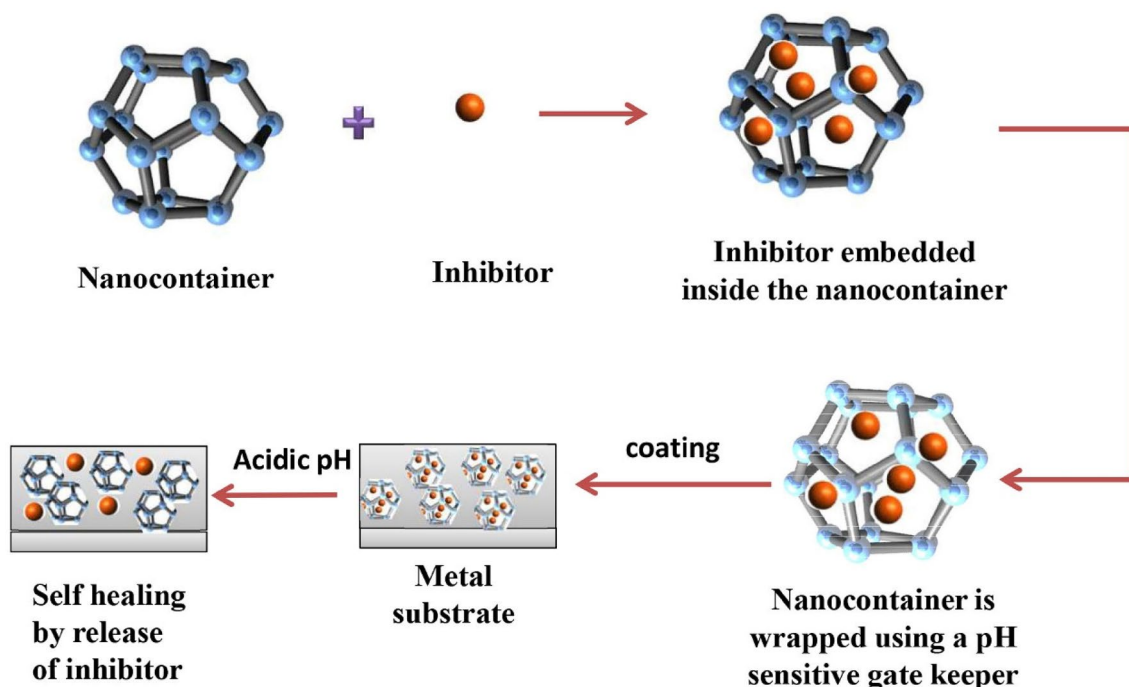
Fig. 5 Mechanism of action of a smart coating
