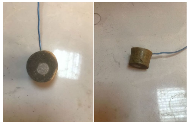
Fig. 2 working electrode consisting of Al–SiC composite
