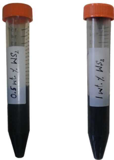
Fig. 1 Representative images of the modified oil containing 0.5 wt% \text{WS}_2 and 1 wt% \text{WS}_2
