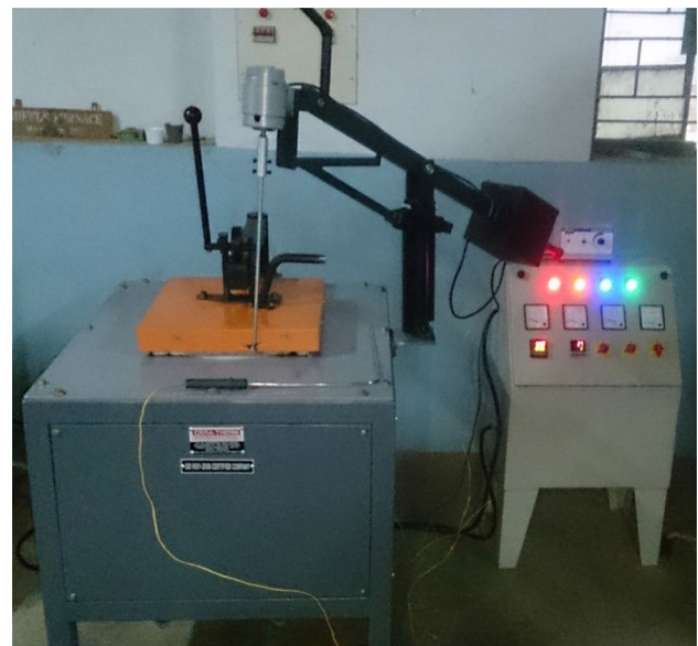
Fig. 1 Stir casting setup used for the composite processing
