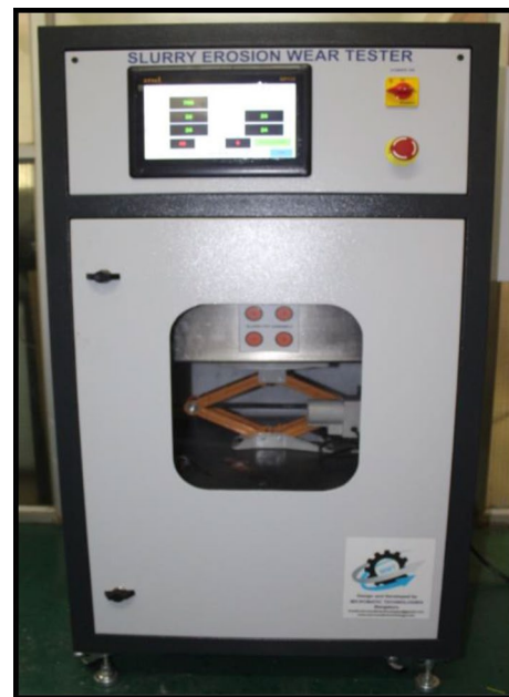
Fig. 1 Photograph of slurry erosion wear tester
