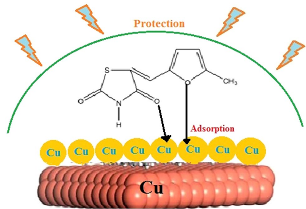
Fig. 23 Diagrammatic illustration of the adsorption of phytochemical derived from plant extract forming a thick defensive layer on the copper surface
