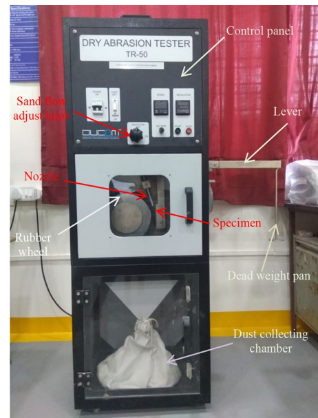
Fig. 5 Experimental setup of dry abrasion tester
