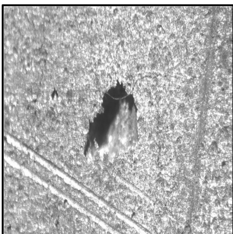
Fig. 6 Optical image of corroded specimen at 5 °C, 24 h
