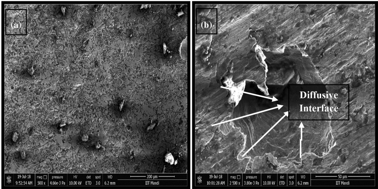
Fig. 16 SEM images of F 304 stainless steel at 5 °C and exposed under 12 h
