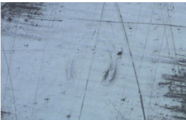
Fig. 17 Optical microscope image of stressed sample at 50 \text{ ms}^{-1} at 60^\circ
