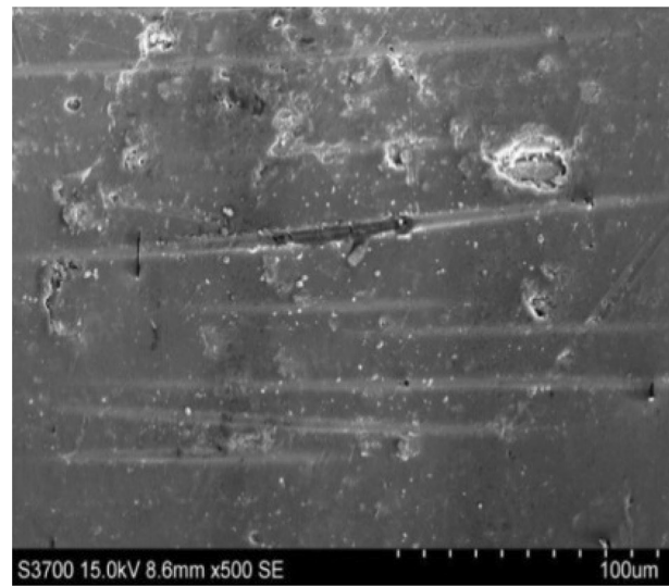
Fig. 11 SEM image of salt water erosion on an unstressed sample at 50 \text{ ms}^{-1} , 45^\circ
