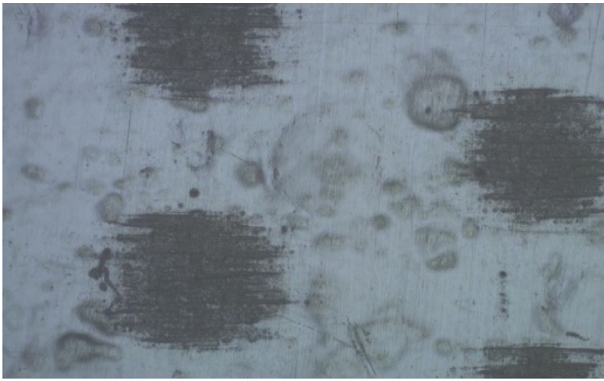
Fig. 16 Optical microscope image of unstressed Sample at 50 \text{ ms}^{-1} , 45^\circ
