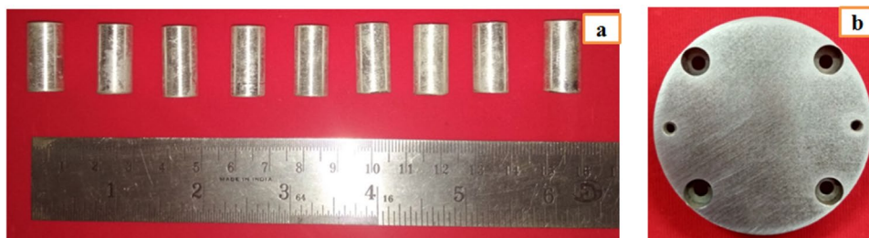
Fig. 2 a Wear specimens and b counterface disc (EN31 steel)
