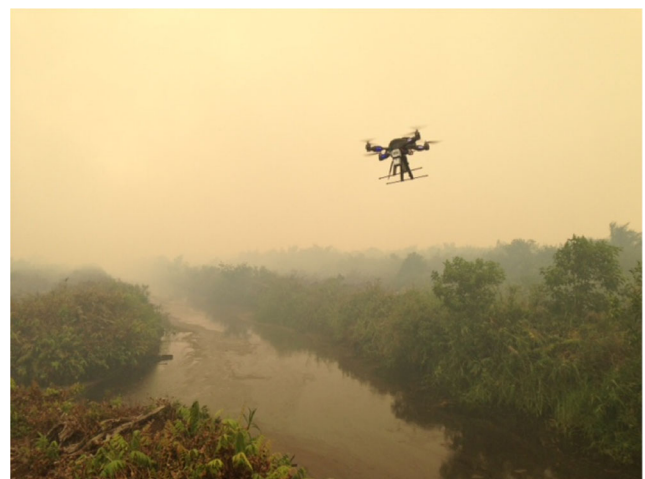
Fig. 1 Remote-controlled drone over South Sumatra during the brief haze event of September–October 2014. Trace gas measurements from the drone are being used to better constrain emission factors from tropical peat burning. (Courtesy of Guido van der Werf, VU Amsterdam)
