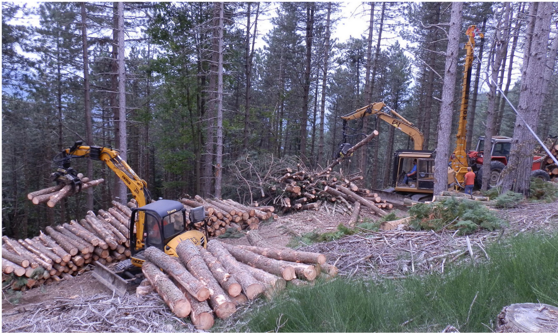
Fig. 1 Integrated harvesting in a yarder operation: after whole-tree extraction, trees are processed into roundwood (left) and energy wood (tops and branches, to the right)
