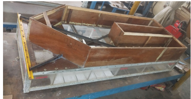
Fig. 3 Fabricated dredge hull model
